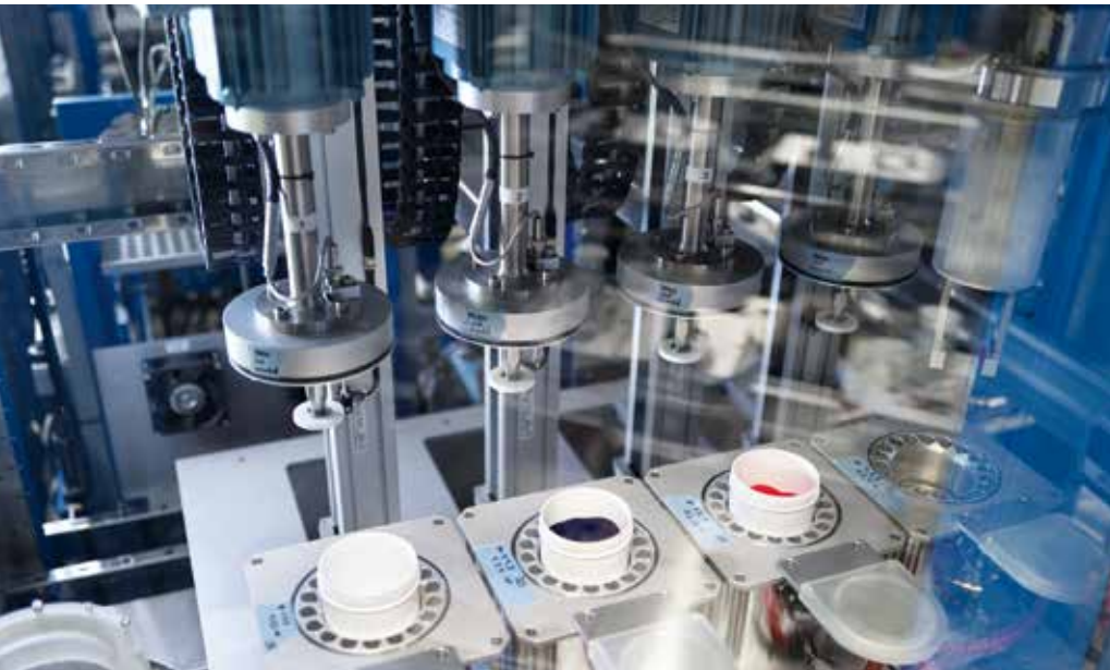
With the fully automated system at BYK in Wesel, 220 samples can be produced and tested in 24 hours in high throughput.
