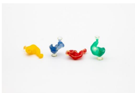
Molds for the production of hearing aids filled with a colored silicone
