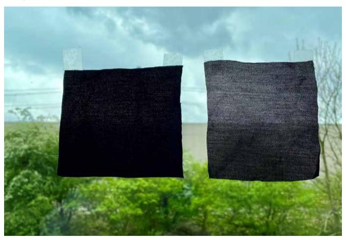
$Light\ transmission\ through\ fabric\ treated\ and\ untreated.$
